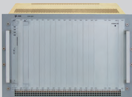
DDN 3001 principle card frame construction
