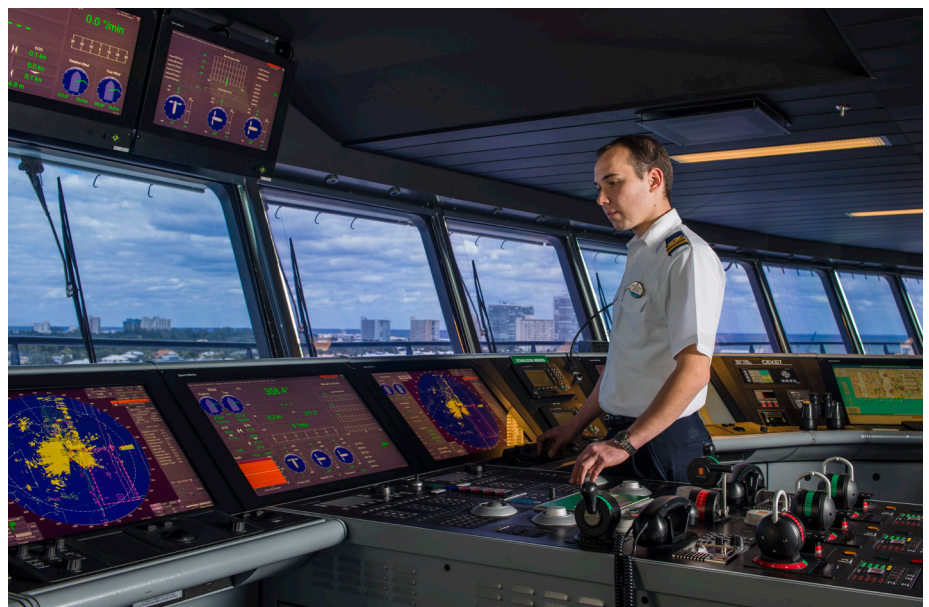
Integrated Bridge System on board the Allure of the Seas
